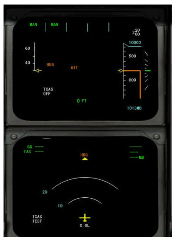
IRS not aligned
